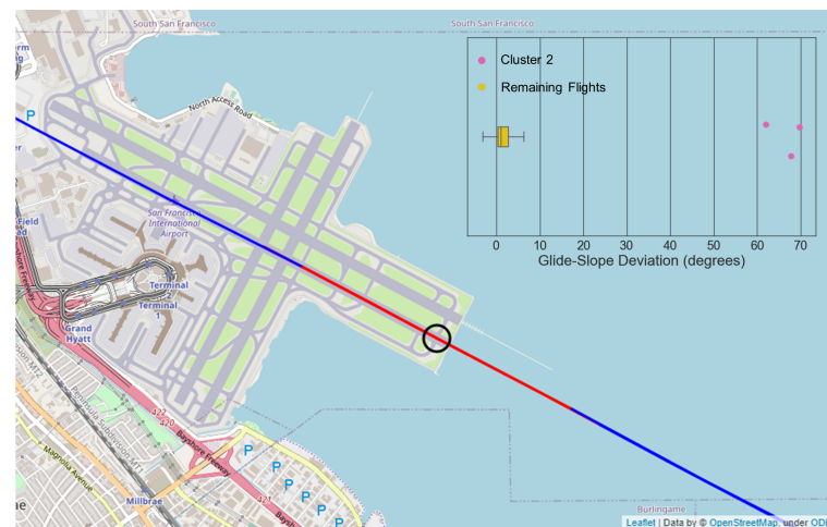
Figure 6. Example of a flight that was placed into the “Other Cluster”. The black circle represents the minimum altitude point prior to go-around. The box-plot in the top right compares the glide-slope deviation of flights in Cluster 2 with the remaining flights. The folium ( http://python-visualization.github.io/folium/ , accessed on 1 September 2021) Python library was utilized to generate the map.
