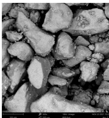
Fig. 3. SEM analysis of Amansea clay before activation (100 μm)
