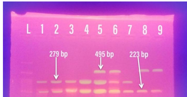
Fig. (1): PCR products of bcsp31 gene (223 bp) specific for genus Brucella , IS711 element downstream of BMEI1162 gene (279 bp) specific for B. melitensis , and IS711 element downstream of the alkB gene (495 bp) specific for B. abortus isolated from the whole blood samples of camels and human in Matrouh Province.
