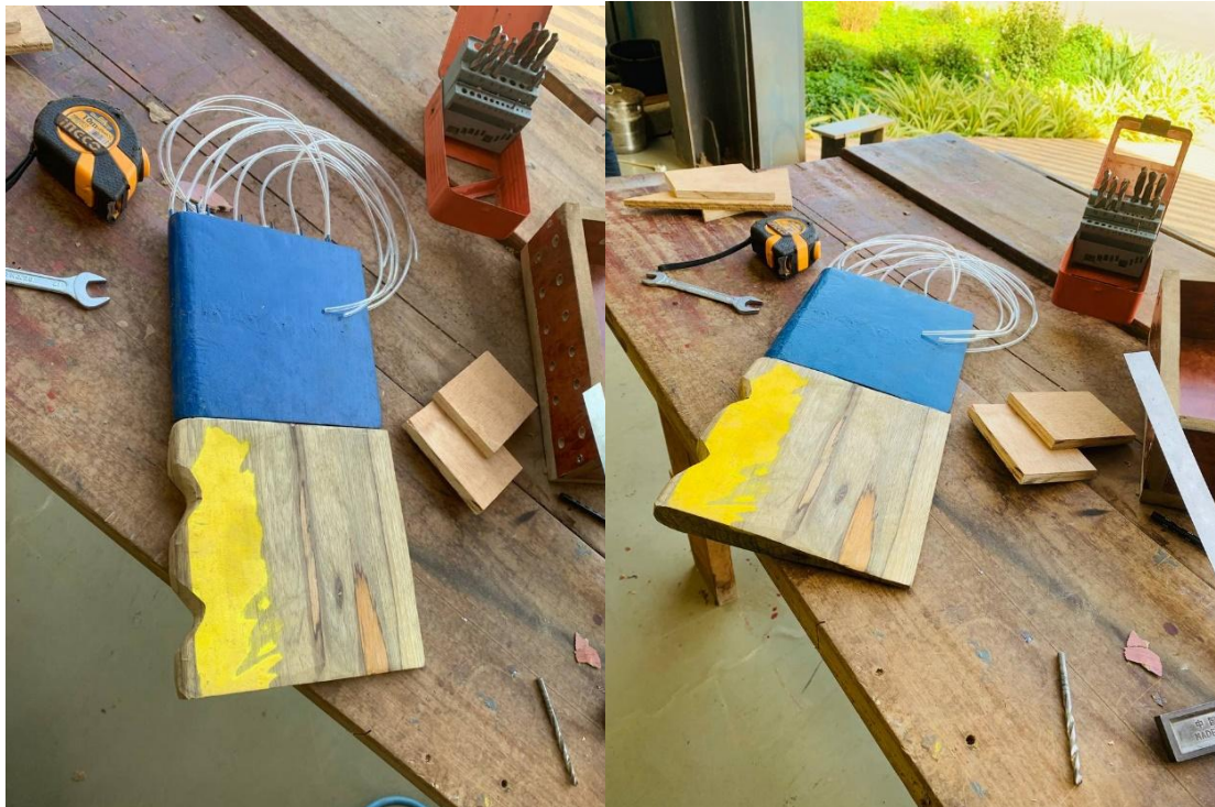
Fig. 16. Hand model of tubercle airfoil and asymmetric airfoil
