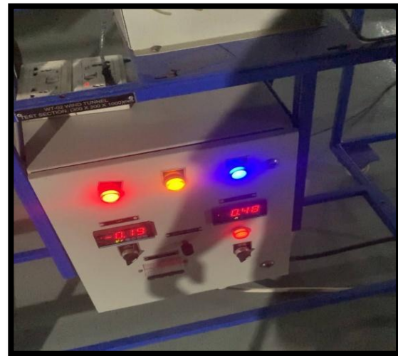
Fig. 17. Wind tunnel results of lift and drag with tubercle airfoil having lift coefficient of 0.4 and asymmetric airfoil having 0.19
