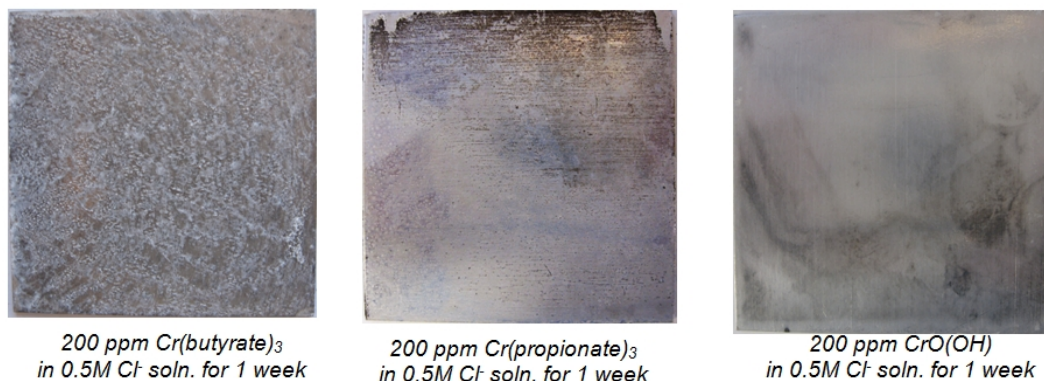
Fig. 7. Images of coupons immersed in various solutions of trivalent chromium compounds
