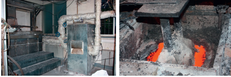
FIGURE 5: Photos of the 2 kA lab-scale heat-exchanging aluminum reduction cell.
