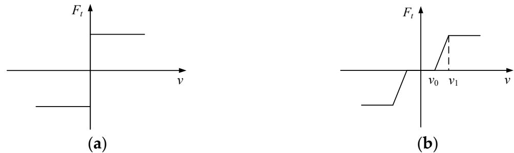
Figure 10. Coulomb friction model and model with modified coefficient introduced: (a) Coulomb friction model; (b) Coulomb friction model with modified coefficient introduced.
