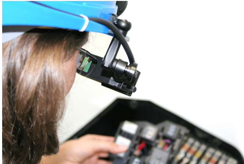
Figure 3. The user is wearing an HMD during the assembly of a control unit. Visual information are displayed in the users field of view.
