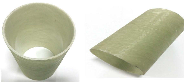
Figure 5. A sample of a fiberglass pipe obtained from unsaturated polyesters of the PN-MA-03 and PN-MA-03A grades.
