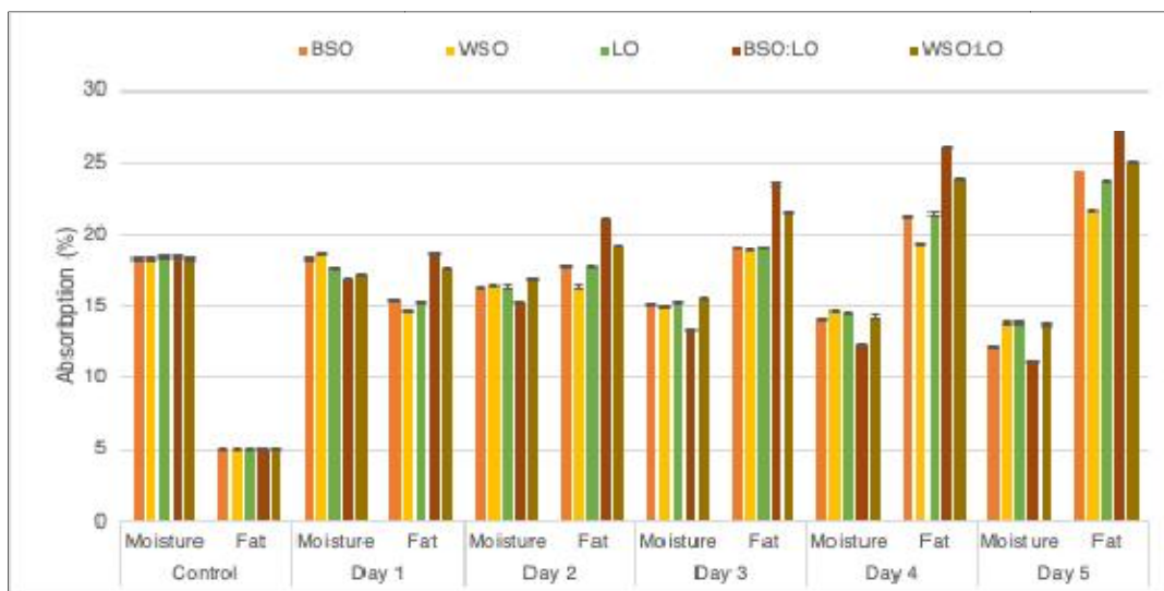
Fig. 5. Effect of frying cycles on moisture and oil uptake during frying of potato chips BSO = Black sesame oil; WSO = White sesame oil; LO = Linseed oil
