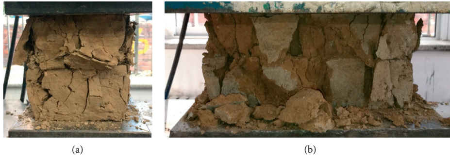
FIGURE 5: Failure modes of stacked half-blocks. (a) Molded adobe. (b) Rammed adobe.
