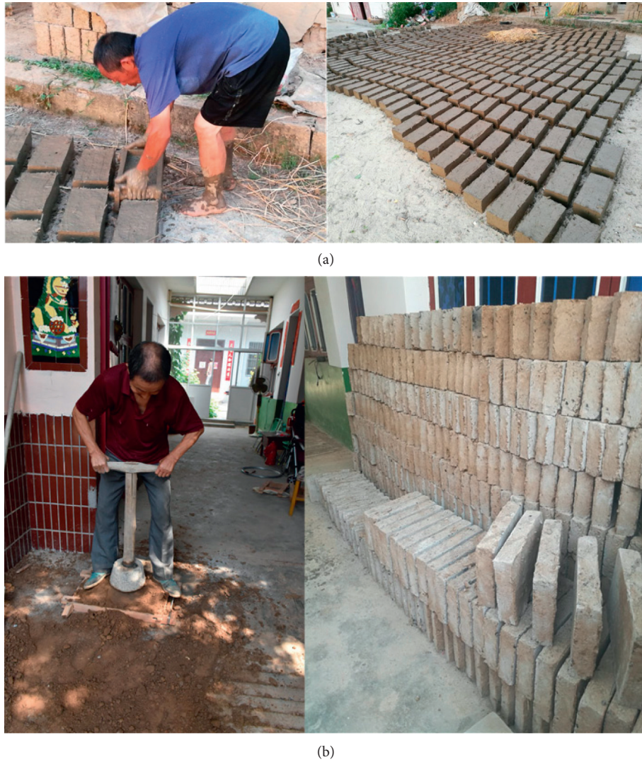
FIGURE 2: Manufacturing process. (a) Molded adobe. (b) Rammed adobe.
