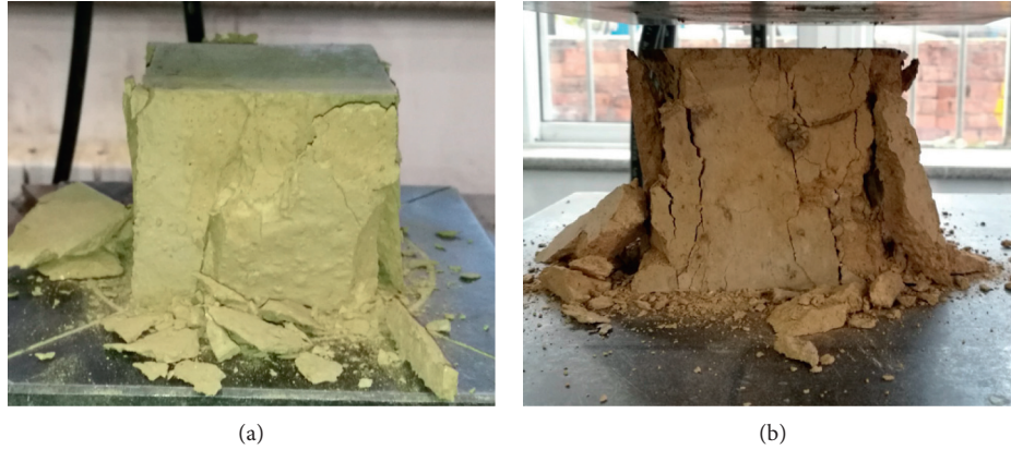
FIGURE 4: Failure modes of cube samples. (a) Molded adobe. (b) Rammed adobe.
